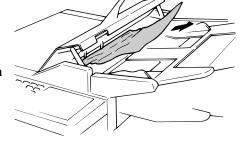
**3** Gently close the scanner cover, making sure both sides are snapped down securely. Then re-try the transmission.
